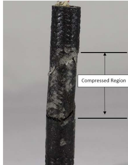
Figure 3. 18: Crushed 13444-13-SG-2 sample after expanding plug test till failure
