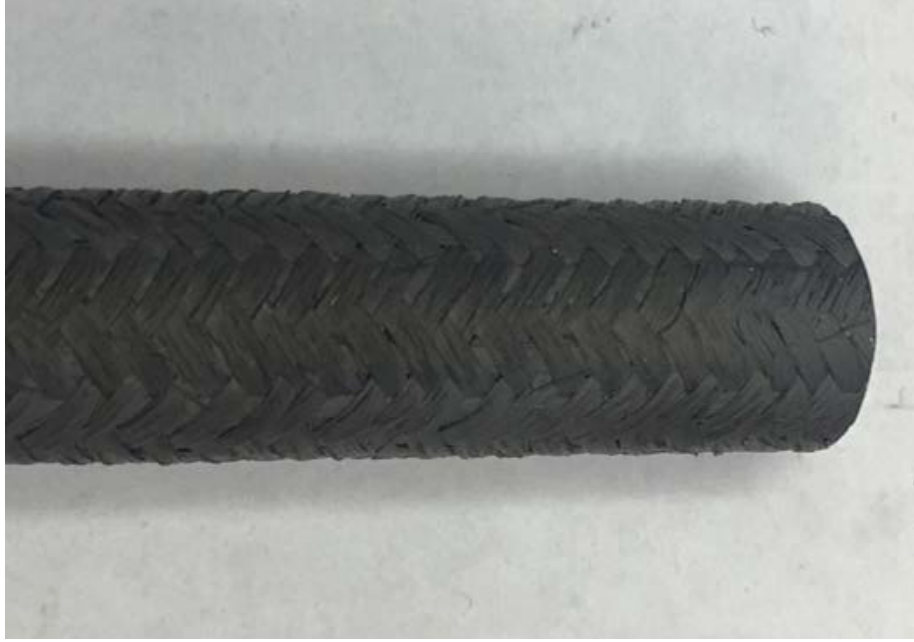
Figure 2. 17: Surface texture for 13444-13-SG-X SiC f -SiC m composite tubing
