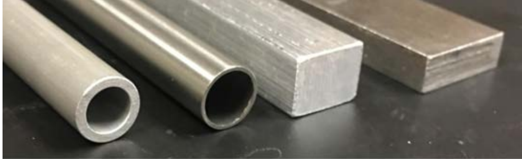
Figure 3.3: Materials used to validate table mounted impulse excitation. (Left to right) Al 2024 Tube, Zircaloy-4 Tube, Al 6061 Bar, and O1 Tool Steel Bar
