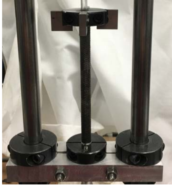
Figure 2.12: Pressure rig mounted IE setup for flexural and torsional testing
