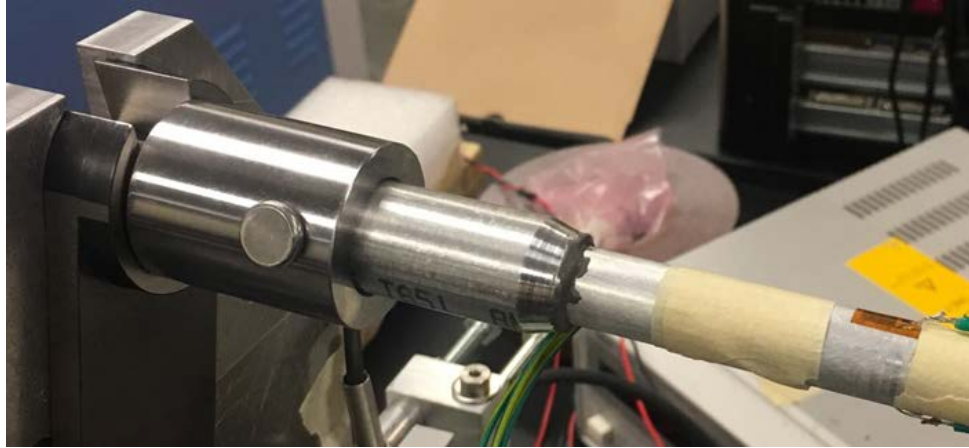
Figure 2.7: Adapter configuration to transmit torsion to the tubular sample
